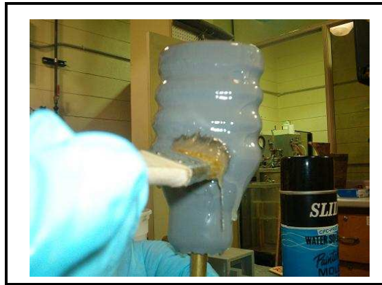
Figure 6: Coating of Polyurethane
