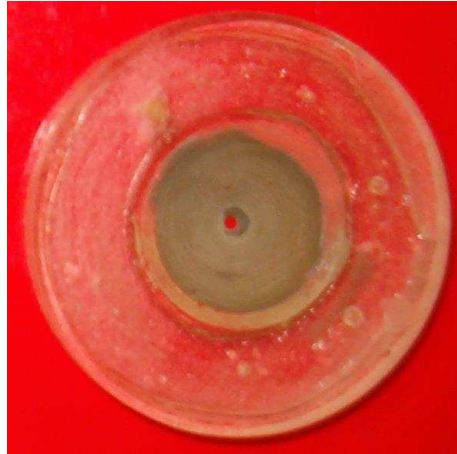
Figure 5. Successful electrodeposition using a silver seed layer
