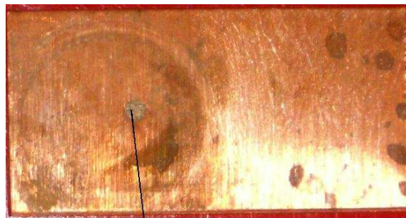
Nickel plating due to direct copper contact
