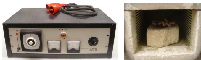
Figure 7. Resistive heating device and furnace
