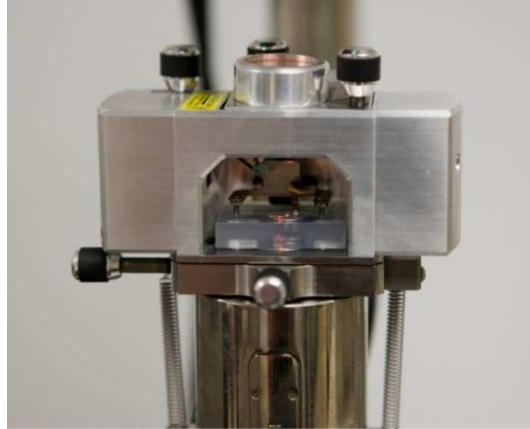
Figure 9. Fluid cell mounted on the atomic force microscope
