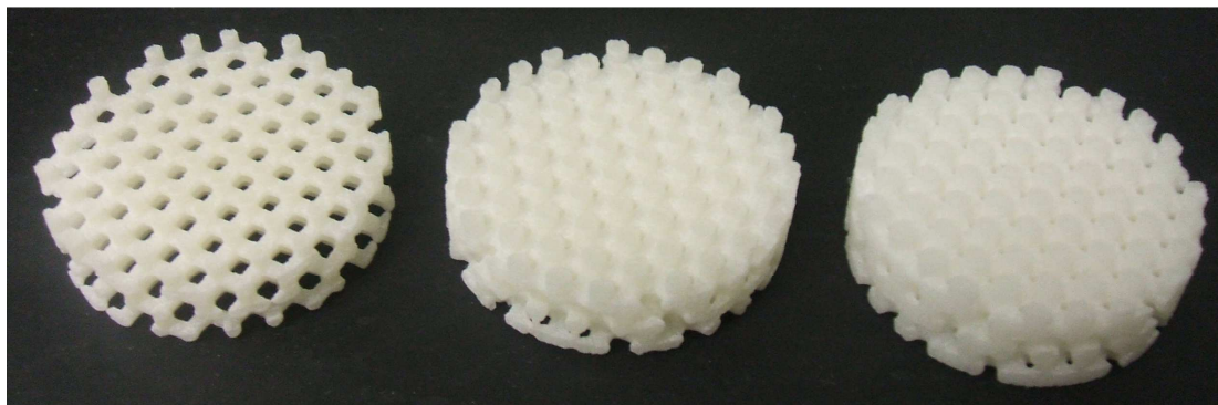
Figure 1. Scaffolds with three different volume ratios. (from left to right: 28%, 44%, 61%).
