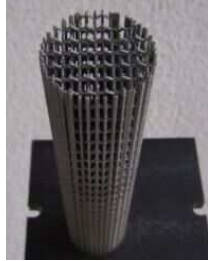
Figure 5. Gradient Tetralattice™ fabricated via selective laser melting.
