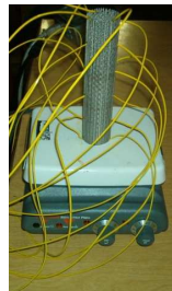
Figures 6. Previous research performed on a gradient Tetralattice™ fin via thermocouples.
